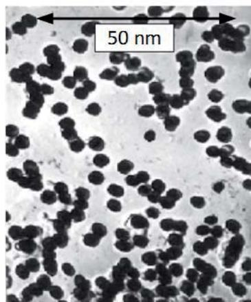
Fig. 4. TEM micrograph of the sample implanted at  $F = 10^{16}$  ions/cm<sup>2</sup>.
