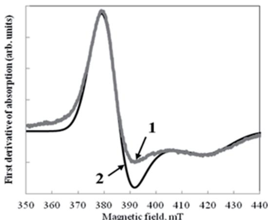
Fig. 3. Experimental (1) and calculated (2) EPR spectrum of  $W^{5+}$  recorded at 300 K for the sample implanted at  $F = 10^{17}$  ions/cm<sup>2</sup>.
