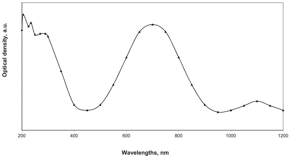
Fig. 2. Optical spectrum in the sample firstly implanted with  $W^+$  ( $F = 10^{17}$  ions/cm<sup>2</sup>) and then  $O^+$ .
